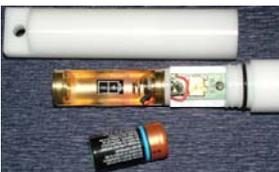
To remove the battery, first open the logger. The battery is held within its casing by the force of a single spring. Press firmly upon the negative end of the battery farthest from the spring and pull it out of the casing.
