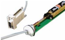
To establish a link between the logger and a PC, open the logger and locate the RJ-11 jack mounted at the end opposite the sensor(s). The supplied RS232 cable has two sizes of plugs. The narrower plug goes into the
