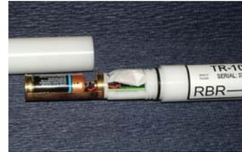
If the logger is closed up in a hotter, more humid environment than the deployment environment and then plunged into cold water, internal condensation can result. Since condensation may cause the circuitry to malfunction, it is advised in such circumstances that, after the logger is set up and before it is closed for deployment, a small pack of desiccant be placed on the battery side of the circuit board above the battery mount.
