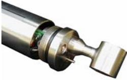
Access to the inner assembly may be obtained by unscrewing the sensor end cap. **Both the battery end cap and the battery carousel must be removed prior to unscrewing the sensor end cap.** Damage to the back plane will result if the wrong end of the logger is opened first.
