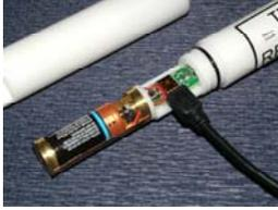
To establish a link between the logger and a PC, open the logger and locate the data port mounted in the middle part of the inner assembly adjacent to the battery holder. The supplied RS232 cable has two sizes of plugs. The narrower plug goes into the logger connector. The other plug fits into the 9-pin serial port on your PC.
