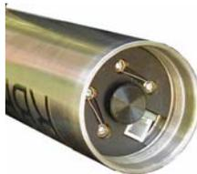
Access to the data port and the battery carousel is gained by removing the end cap opposite the sensor end of the logger. It may be unscrewed by hand or by using a rod inserted into the mooring line hole for leverage. The end cap does not unscrew completely until the O-ring is clear of its mating surface in the body. This ensures that it will not eject at high speed should the interior of the logger become pressurized.
