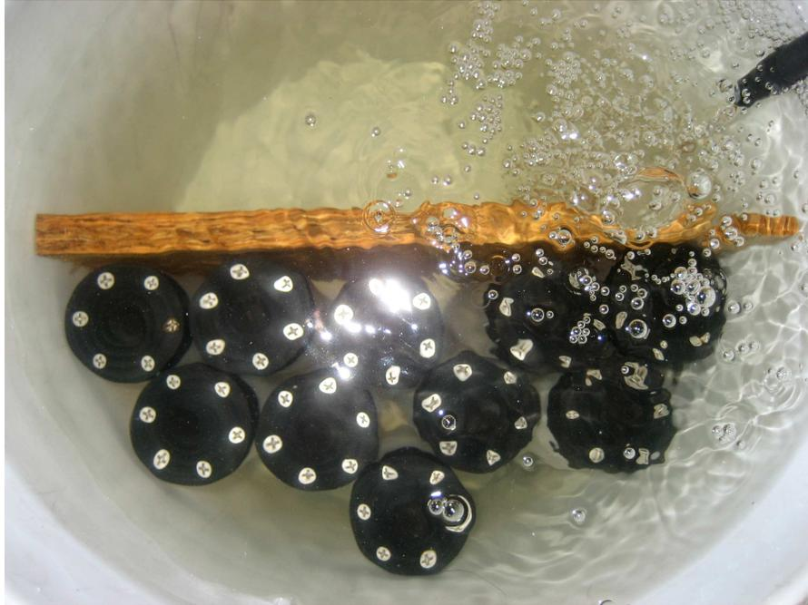
Record measurements for several hours or a day but in any event long enough for the miniDOT temperature to come to equilibrium with the water. During the experiment find the local air pressure, either from measurements or from a local weather station. Watch out... weather stations often report barometric pressure referenced to sea level. You must determine the barometric pressure at your elevation.
