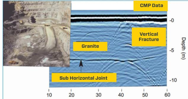
Detect changes in rock type, fractures, faults and joints for safety and resource development in underground mines.
