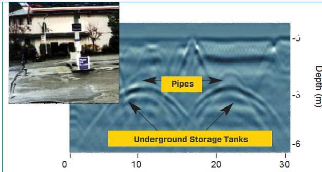
Map depth to bedrock, detect sinkholes, locate underground storage tanks (USTs). Drainage systems on golf courses and farms can also be located.
