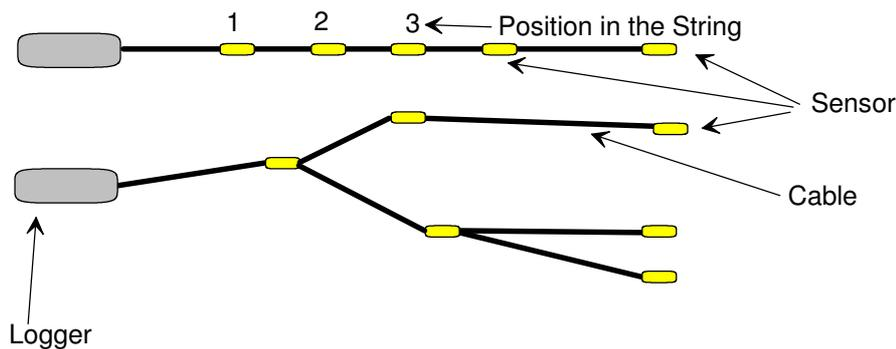
The total cable length should be kept less than less than 20-50 meters (depending on the cable type and number of sensors)!
