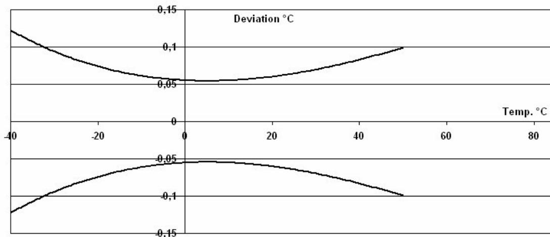
The platinum based high precision sensors itself are optimised for the temperature range  $-10^{\circ}\text{C}$  to  $+20^{\circ}\text{C}$ , but it is suitable for the range  $-40^{\circ}\text{C}$  to  $+85^{\circ}\text{C}$  with reduced accuracy. The long term stability of the sensors, if operated in the range  $-20^{\circ}\text{C}$  to  $+40^{\circ}\text{C}$  is not significant. The resolution of the sensors are  $0.01^{\circ}\text{C}$ .
