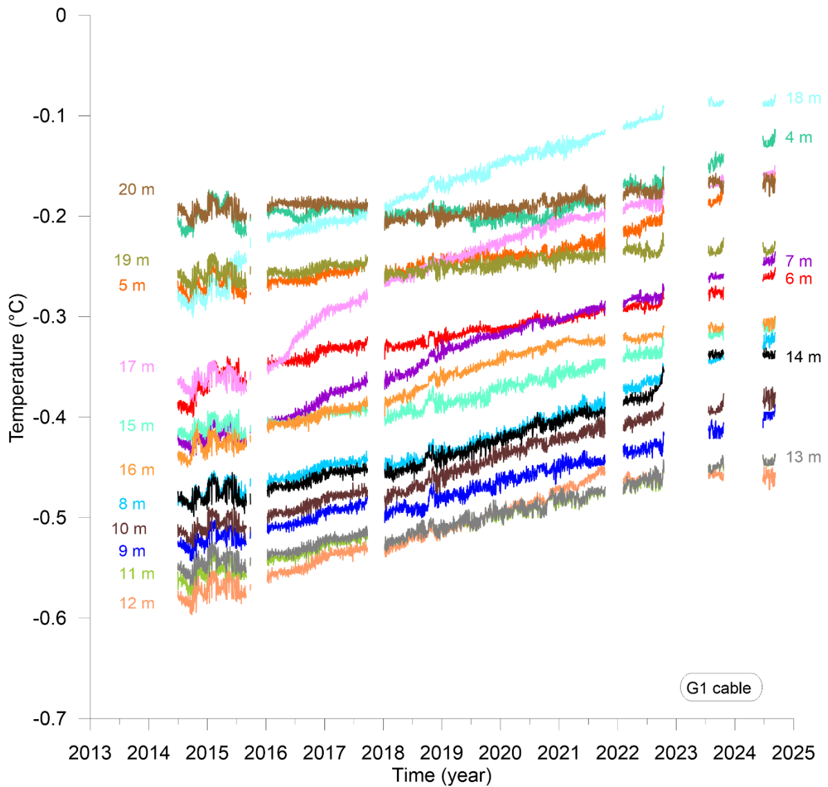
Figure 7: Time series of ground temperatures measured with thermistors at depths from 4 to 20 m of the G1 thermistor cable on the top of the SB lithalsa. The thermistors at depths of 7, 17, and 18 m exhibit erratic behavior showing a significantly higher increase in ground temperature after the interruption in 2015-2016 than the other thermistors.
